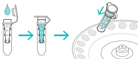
Figure 3. Orientation of the Amicon Ultra-0.5 mL Centrifugal Filter Unit.
