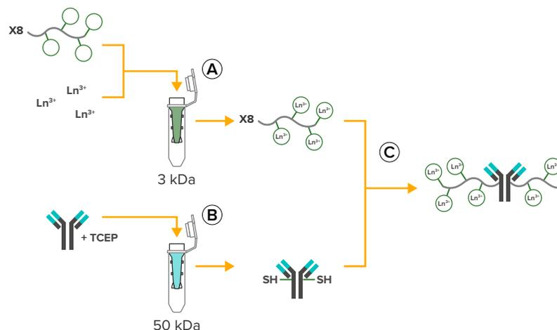
Figure 5. This procedure involves first loading the X8 polymer with Ln metal solution (A) and partially reducing the antibody (B), then conjugating the antibody with the Ln-loaded polymer (C).
