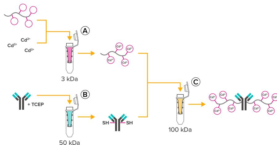
Figure 1. This procedure involves first loading the MCP9 polymer with Cd metal solution (A) and partially reducing the antibody (B), then conjugating the antibody with the Cd-loaded polymer (C).
