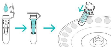
Figure 7. Orientation of the Amicon Ultra-0.5 mL Centrifugal Filter Unit
