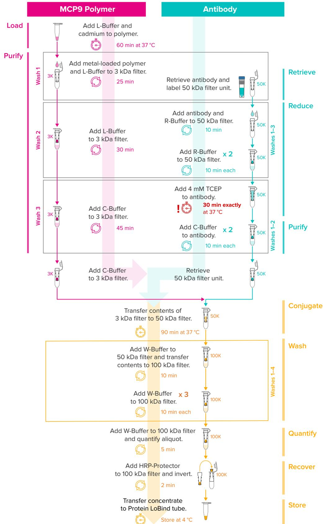
Figure 2. Overview of the Maxpar MCP9 Antibody Labeling procedural workflow
