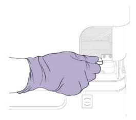
**3** Load the slide onto the stage and close the sample window.
